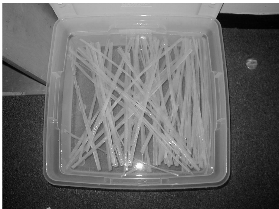
Figure 8. The pounded strips are soaked for three to six days to remove sugars from the plant.
