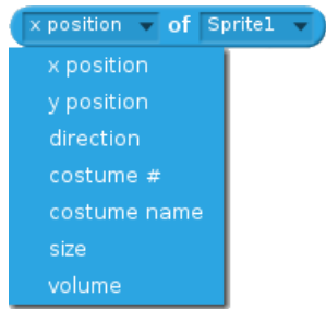
Figure 2: Accessor method block for Scratch sprites, with a dropdown to select the appropriate property. The shape of the block indicates it is a “reporter” block, and that it can be used as an input to another blocks (e.g., the “say” block).
